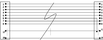
Figure 4-24: PUT Miswired – reversed
