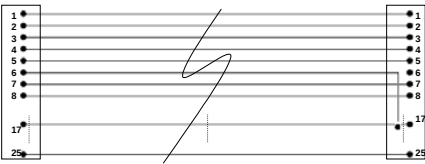
Figure 4-6: PUT Miswired – reversed
